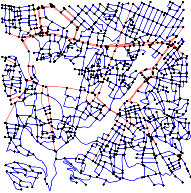
Fig. 1: Partial road network for the city of Bursa, TURKEY. From the city center, the nodes within a bounding box of 1000 meters are included. Red color denotes one-way traffic.
